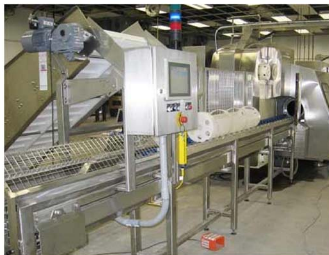
Gridpath's peripherals work included the operator panel that displays validation results. The white basket in the background is loaded with product before being conveyed into the pressure chamber (right). Source: Gridpath Solutions Inc.
